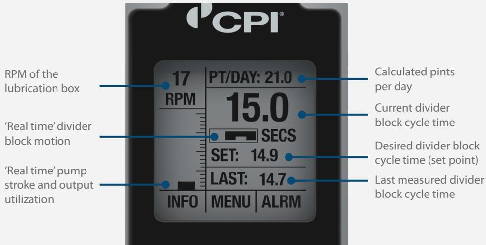
EOS has fully interactive interface built into the unit. Control your parameters from the EOS or from your modbus connected PLC.
